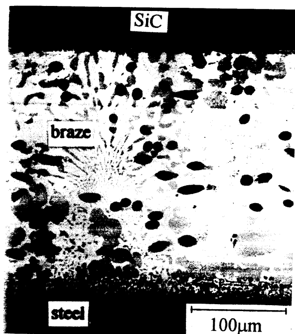
Fig. 3. Polished cross-sectional microstructure of the composite brazing layer between SiC (top) and 304 stainless steel (bottom). The carbon fibers were uniformly distributed.
