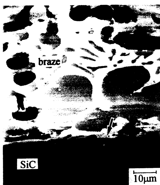
Fig. 10. SEM backscattered electron image of the brazing layer near the SiC/braze interface (with carbon fibers).
